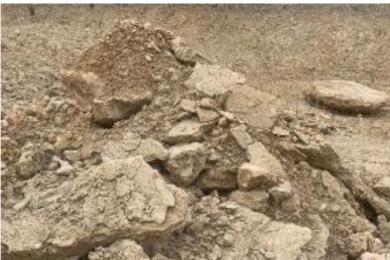
Figure 7 Typical 100mm Road Base Material
