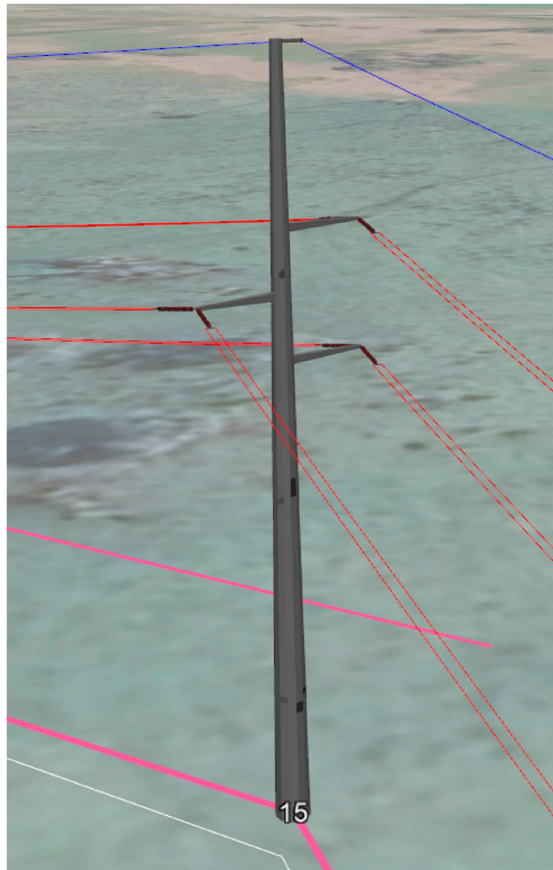
STRAIN POLE STRUCTURE 36.0M HEIGHT 7 NO OFF BASE PLATE AND ANCHOR BOLTS
